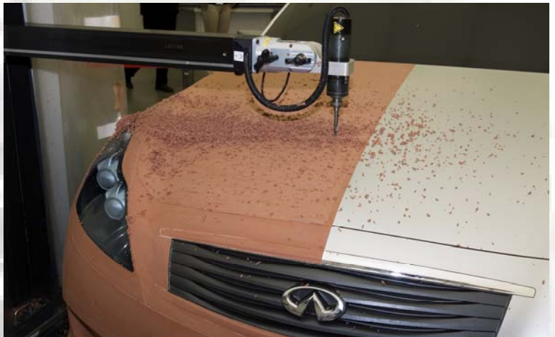
Simplified automatic cutting machine
